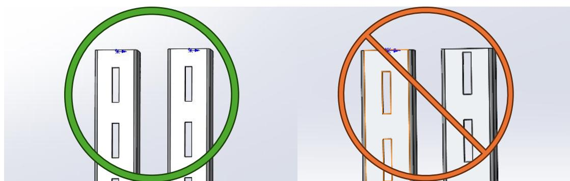
4. Position case brackets (**D,E,F**) in standards. Place the bracket hooks in 2<sup>nd</sup>, 5<sup>th</sup>, and 6<sup>th</sup> slots from the bottom.
