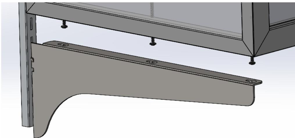
6. Install the provided clips (**G**) for the top of the case. These clips should slide behind the standards, with the hole in the clip positioned over the case and ready for the provided screw. Use a 7/64" Drill bit to predrill the holes in the frame of the display case, careful not to drill more than necessary. Ensure the case is firmly against the standards before driving the screws (**B**).
