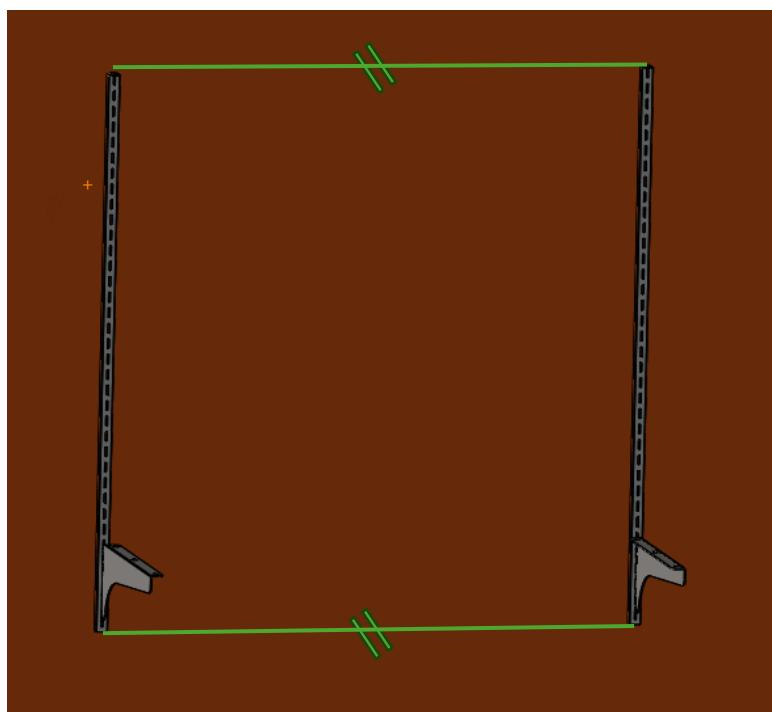
3. Securely attach the standards to the wall using appropriate hardware suitable for the wall's construction. For walls built with 2x4 framing, use the provided stud screws (A). Refer to local building codes for guidance on hardware suitable for other types of wall construction.
